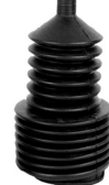
Axle Bellows, Wheel Side- (Ø10 - Ø40) R19 I, R21, CLIO I, EXPRESS, MASTER
